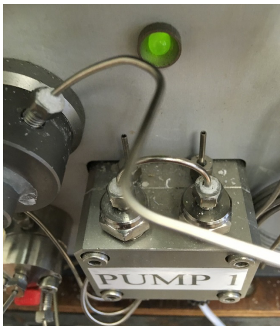
Figure 18 Picture showing solid (presumably mandelic acid) at the junction of the HPLC pumps.
