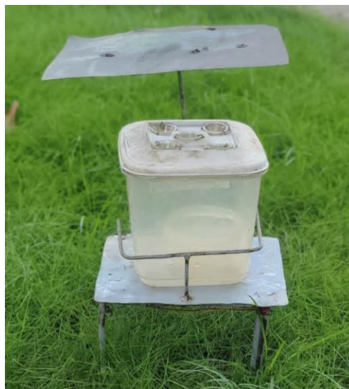
Figure 4.7: Lindsay domestic fly traps were affixed to metal stands for fly sampling at the toilets.
