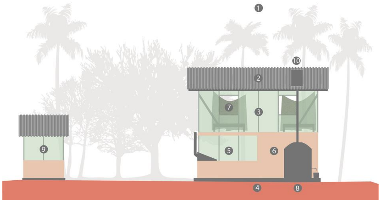
Figure 1.5: Components of the Star home. Where 1) building orientation, 2) lightweight roof, 3) facade openings, 4) raised concrete floor, 5) screened indoor cooking area, 6) lockable storage area, 7) raised sleeping area, 8) water harvesting system, 9) fly-proof latrine and 10) solar power, (Mshamu et al., 2022).
