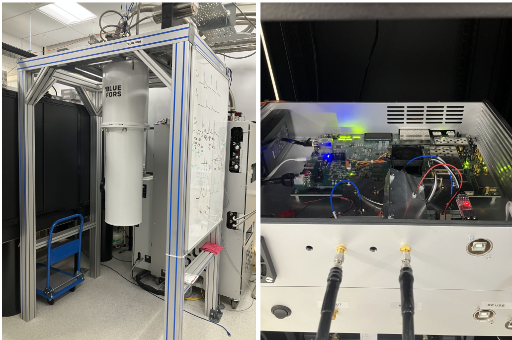
Figure 5.3: Left shows a BlueFors dilution refrigerator. Achieves sub-Kelvin temperatures by pumping liquid helium throughout the system to cool the MKID, as described in Sec. 2.3. Right shows the Xilinx board used to generate and receive the microwave tones used for reading out the MKID devices.
