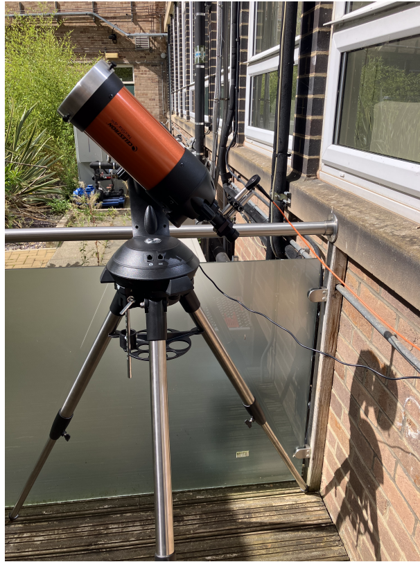
Figure 6.19: The Celestron Nexstar Telescope used to observe the Sun, with the 3D printed fibre attachment on the rear of the telescope. The orange fibre was fed from the telescope to the KIDSpec Prototype through the lab window.
