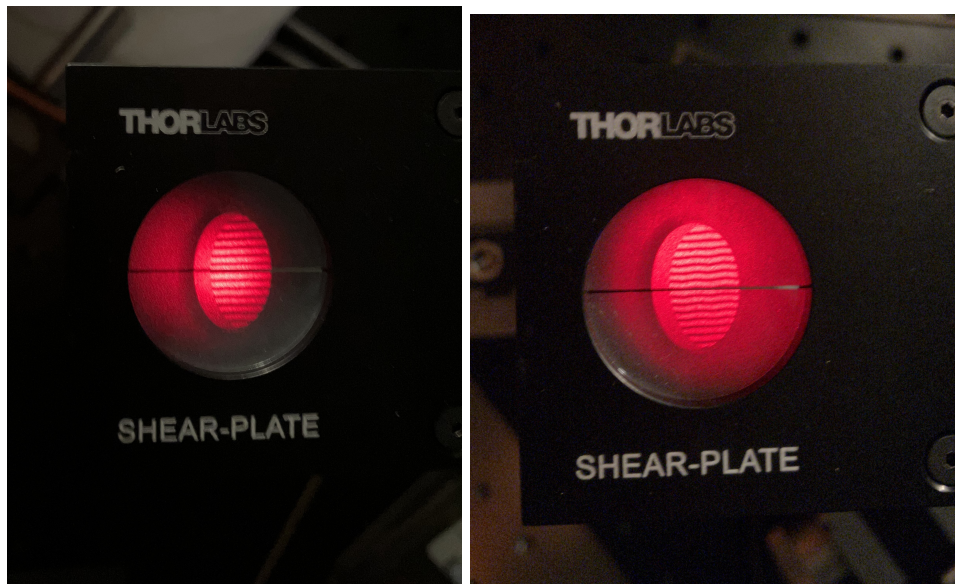
Figure 6.7: Pictures taken of the shear plate from the SI100 when a 633nm laser was used. Left is the collimation result for the 76.2mm focal length OAP mirror. Right shows the collimation for the 203.2mm focal length OAP mirror. Because the pattern is clearly vertical along the line included on the shear plate, both were assumed to be collimated.
