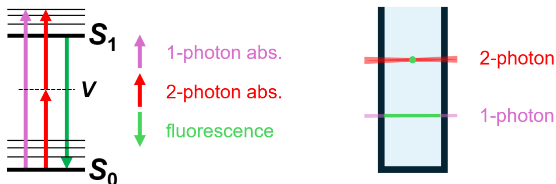
Figure 1.25. A Jablonski diagram depicting multiphoton excitation where hv_1 = 2hv_2 , and V is a virtual transition state ( left ). Schematisation of the effect of fluorescence arising in a cuvette from 2-photon and 1-photon excitation (1PE): excitation volume of 2-photon excitation (2PE) is a small volume ( right ).
