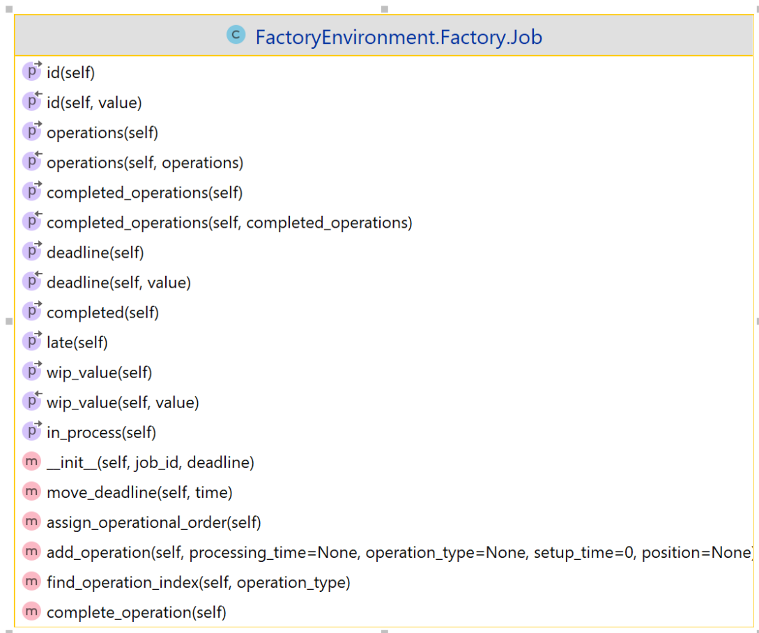
Figure 9: UML diagram for the job class including class methods and properties.
