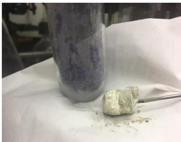
Figure 3.8. (i) Purple (3) /SiO 2 prior to exposure to atmosphere (ii) Green (3) /SiO 2 after exposure to air
