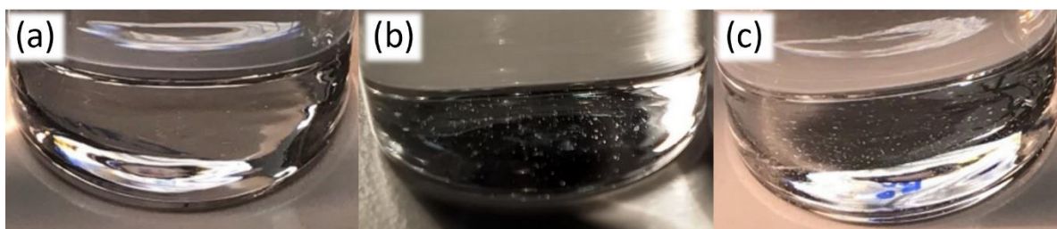
Figure 4.22: Visible glycine crystallization in the seeded binary ethanol/water solutions containing 0.60 mass fraction ethanol and \frac{c}{c_{sat}} = 1.30 after (a) 1 hour for \gamma -glycine crystallization due to seeding with the 0.25 water mass fraction STF with \frac{c}{c_{sat}} = 1.30 , (b) 10-20 minutes for \beta -glycine crystallization due to seeding with the 0.25 water mass fraction STF with \frac{c}{c_{sat}} = 2.10 and (c) 1 hour for \alpha -glycine crystallization due to seeding with the 0.40 water mass fraction STF with \frac{c}{c_{sat}} = 1.30
