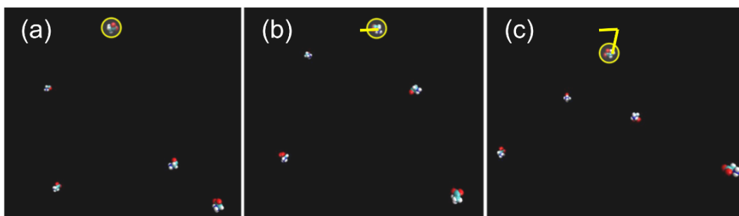
Figure 6.3: Snapshots from a simulation displaying diffusion in an STF containing water, octanol and ethanol mass fractions of 0.15, 0.50 and 0.35, respectively. (a), (b), and (c) were captured after 0 ns, 1 ns, and 2 ns, respectively. A molecule has been highlighted to show its trajectory.
