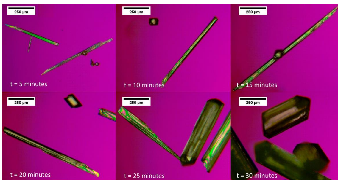
Figure 4.14: Optical micrographs showing the solution-mediated phase transformation of \beta -glycine to \alpha -glycine within 30 minutes for the \frac{c}{c_{sat}} = 2.4 system.
