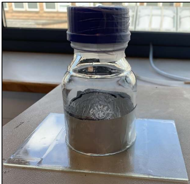
Figure 3.1: 89.1 mm * 89.1 mm * 300 \mu m 2-layer film with solvent well attached.
