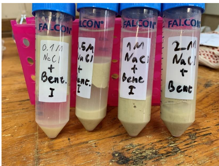
Figure 9. Attempted Bentonite clay gelation, without agitation, in different strength NaCl solutions.
