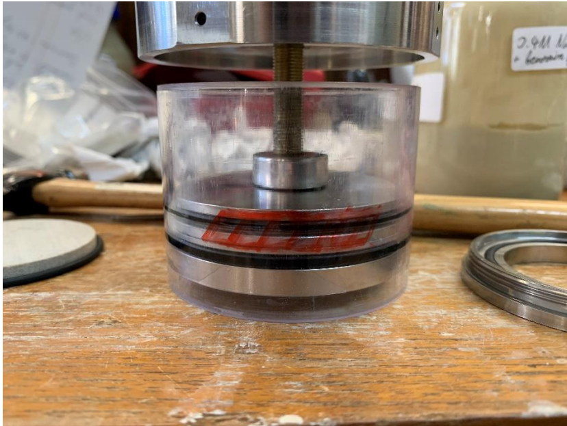
Figure 13. Press making contact with the sample holder.
