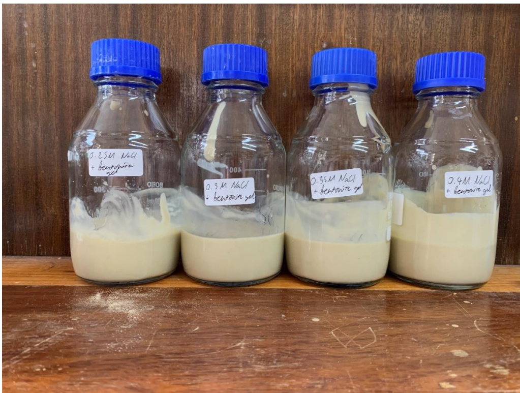
Figure 10. Gels prepared using a blender to induce agitation.
