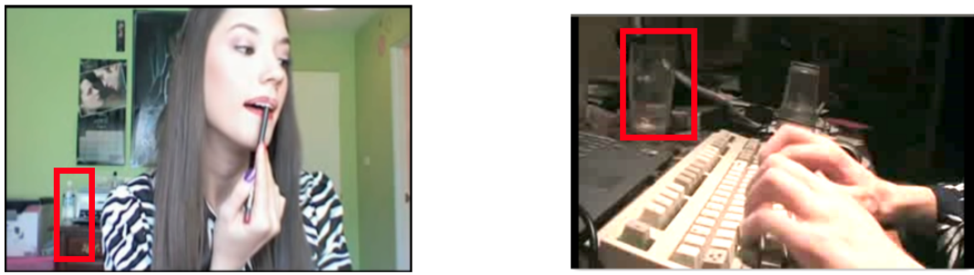
Figure 3.4: Some of false detections cases: (Left) Drinking bottle is detected as the main object for interaction instead of lip brush. (Right) A Cup is detected as the main interacting object instead of the keyboard.
