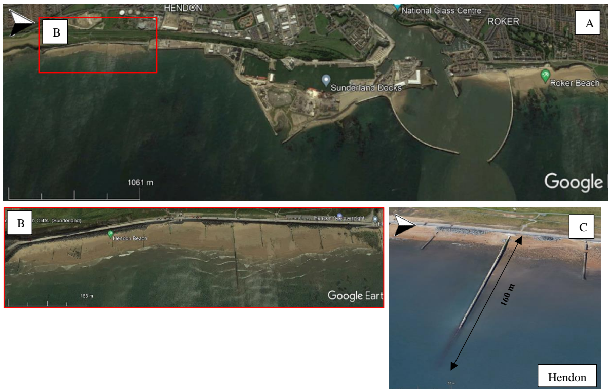
Figure 24: 2021 satellite imagery of (A) coastline from Roker beach to Hendon beach showing Sunderland docks preventing southward sediment drift from Roker beach to Roker Cove beach and Hendon beach. (B) Hendon beach divided into ~75 m sections by 12 wooden groynes. (C) 160-metre-long sewage pipe extending from Hendon beach into the North Sea.
