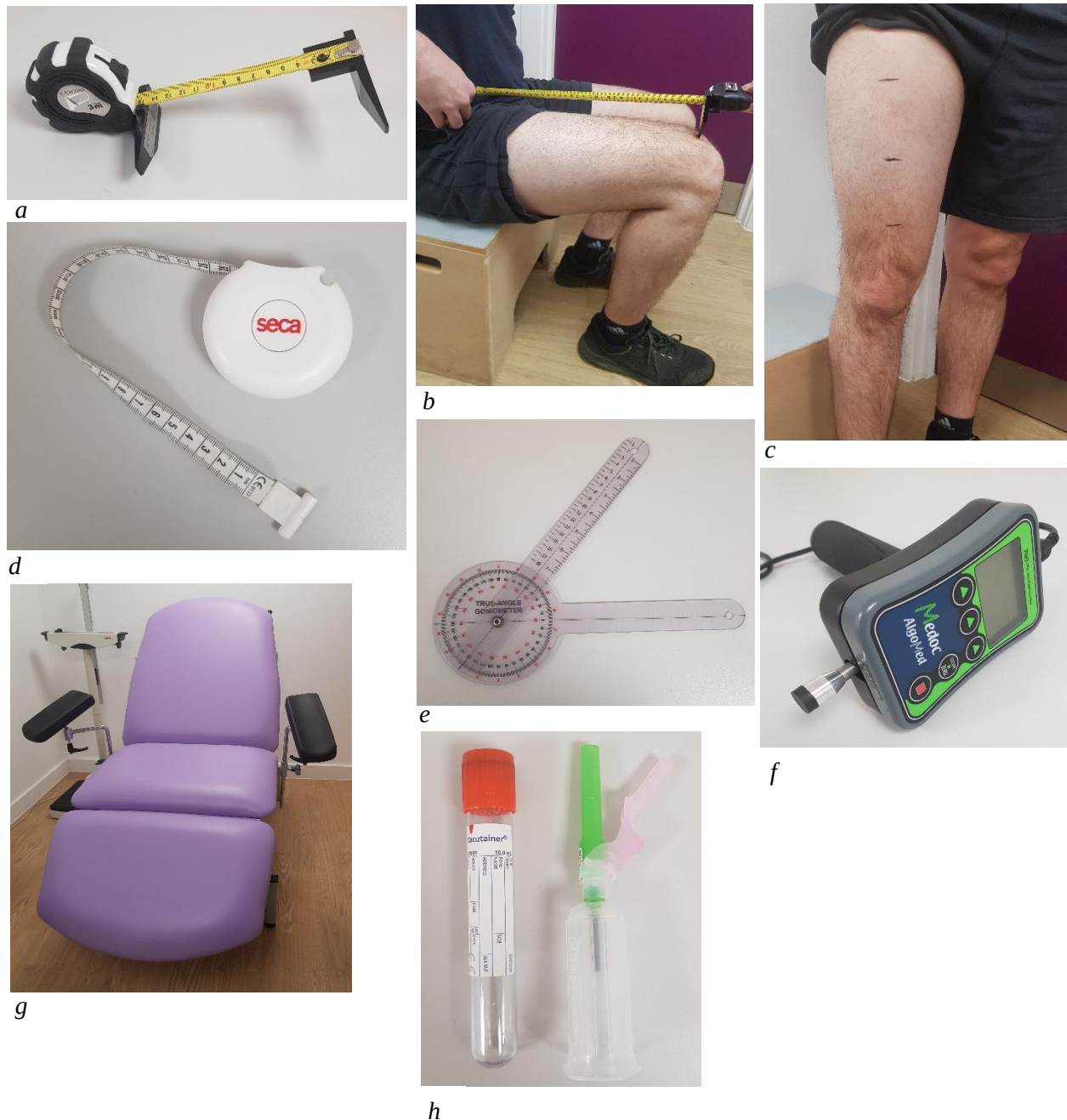
Figures A4.a–h. Materials used for the assessment of exercise-induced muscle damage: a. segmometer, b. seating positioning during measurement of the trochanterion-tibiale lateral site, c. marked points at the mid, lower-, and upper- quartiles of the trochanterion-tibiale lateral site, d. anthropometric tape, e. goniometer, f. pressure algometer, g. phlebotomy bed, h. 10 mL reagent-free vacutainer (left) and 21 g vacutainer safety needle and holder (right).
