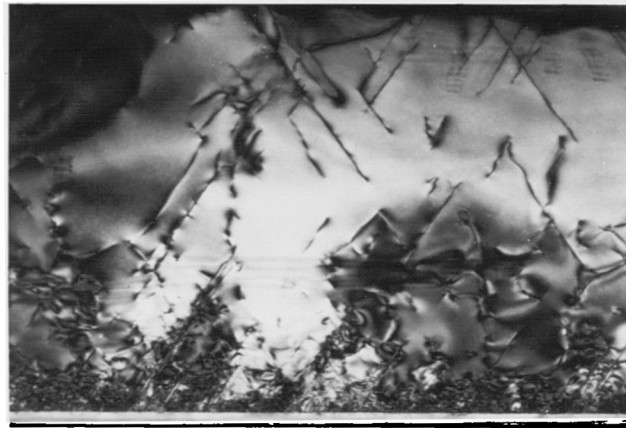
Figure 5.5 — An XTEM micrograph of a layer of CdTe grown at 325°C on {100} GaAs
