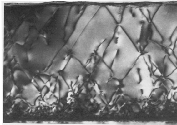
Figure 5.21 — XTEM micrograph of a ZnTe layer grown on \{100\} GaAs at 350^\circ\text{C}
