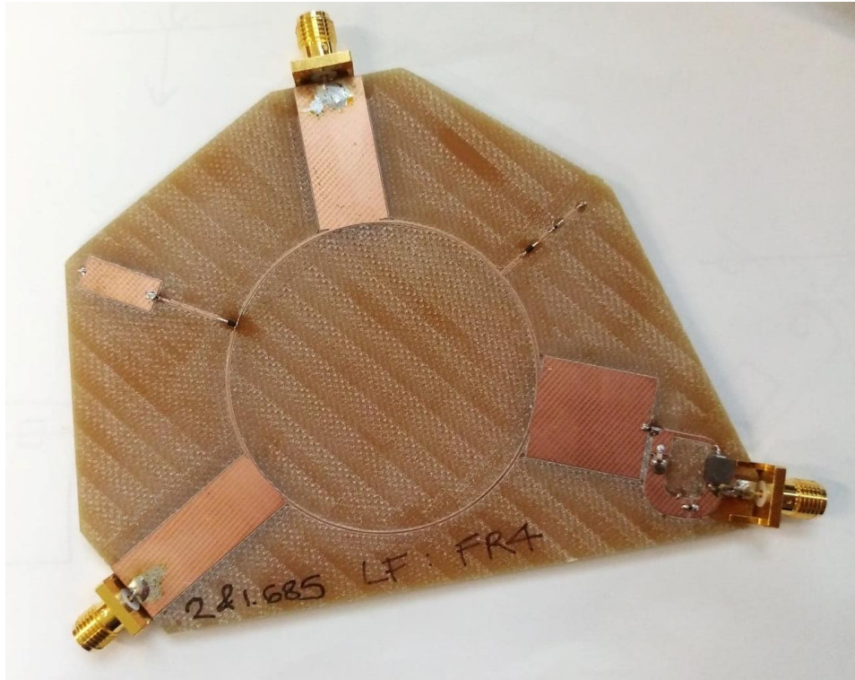
Figure 103: Fabricated 2 GHz mixer on FR4 substrate. Design shown in Figure 101.
