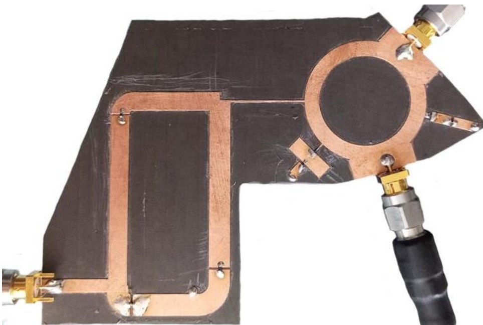
Figure 111: Fabricated 20 GHz mixer on RT/Duroid 5870 substrate. Design shown in Figure 109.
