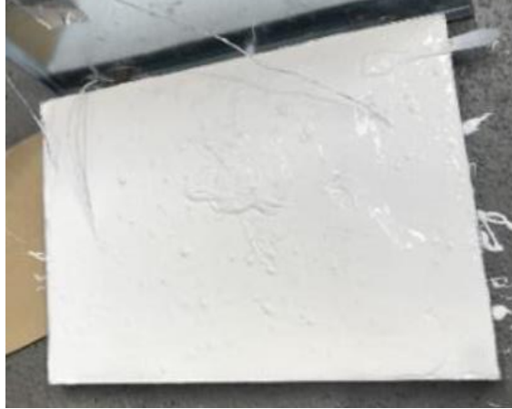
Fig. 4.5 Photo of the battery heat source covered by the silicon paste.
