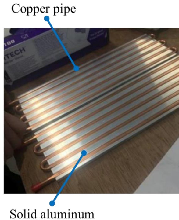
Fig. 4.6 Photo of the battery cooling module.
