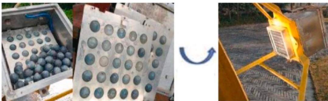
Fig. 2.11 Macro-encapsulation of PCM example: using PCM-encapsulated spheres [130].
