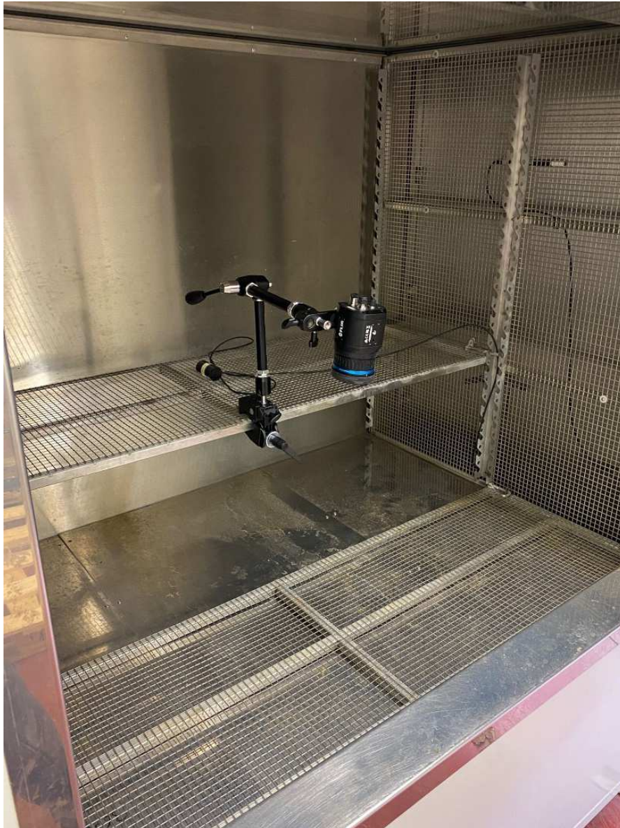
Figure 2.1: Infrared video thermography (IRVT) experimental setup. A FLIR A700-EST was mounted on a Manfrotto Magic Arm and Super Bracket. The mounted camera was clamped onto a shelf inside a Weiss Technik Fitotron Modular Plant Growth Chamber. Trays of plants were placed onto the floor of the chamber directly under the camera lens for imaging.
