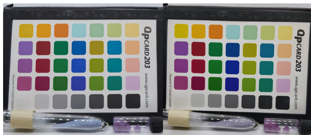
Figure 2.19 Neodymium chloride samples illuminated by broad-spectrum white LED illumination photographed with different cameras: Sony a6000 (left), and Oneplus 5 featuring a Sony IMX 398 sensor (right). The in-camera white balance was set from the white tile on the QP203 colour standard card.
