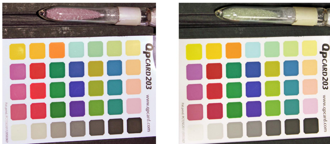
Figure 2.3 A single sample of anhydrous neodymium chloride under sunlight (left) and fluorescent lighting (right) including a QP 203 82 colour standard card for reference. Photographs were taken using a Canon EOS 60-D digital camera.
