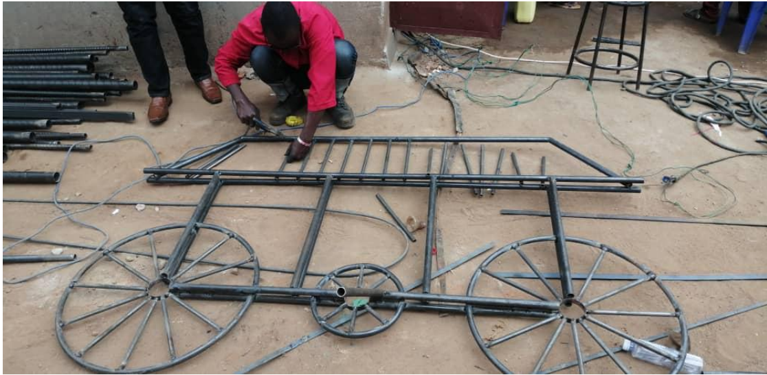
Plate 53: The process of welding the covid bikes, Katwe industrial area, July 2020
