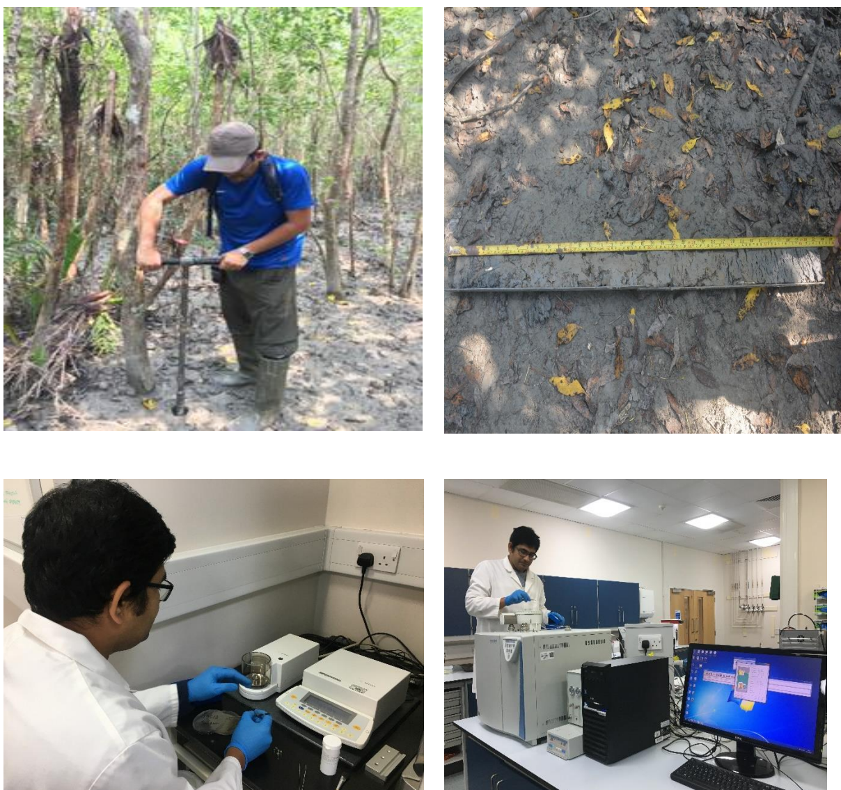
Figure 3.8: Sediment collection and the determination of SOC in the laboratory. Top-left: sediment core collection, top-right: sediment core, bottom-left: weighing sediment sample for measuring organic carbon, bottom-right: loading sediment sample in the CHN analyser.
