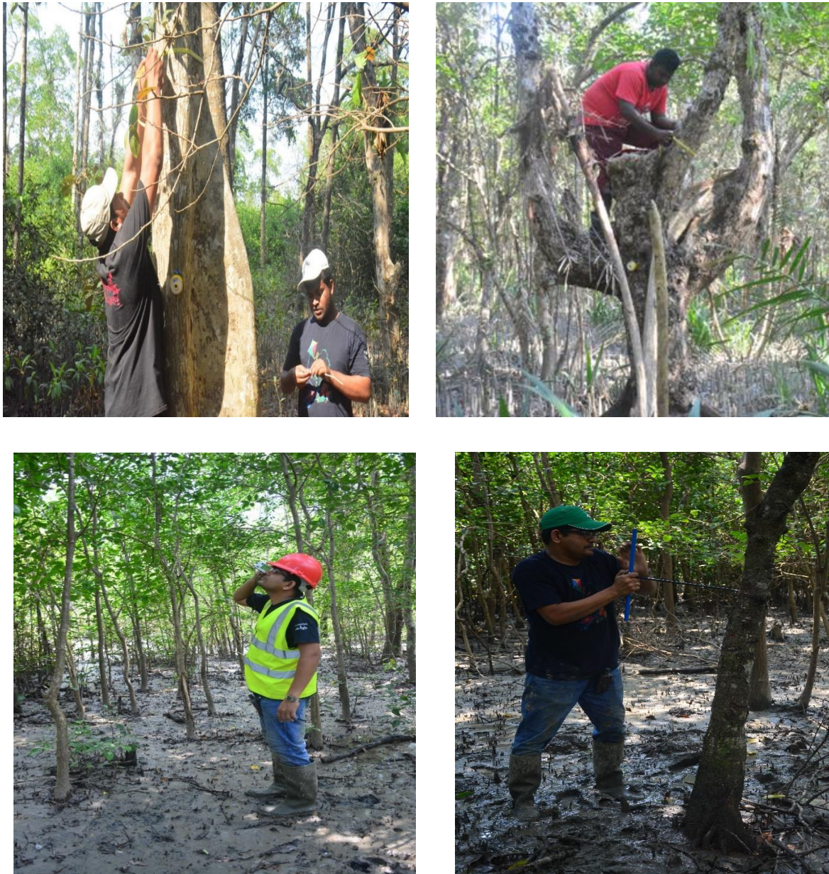
Figure 3.7: DBH and height measurement and collection of wood core. Top-left: DBH measurement by diameter tape above buttress, top-right: DBH measurement above forking, bottom-left: height measurement with a Vertex-III hypsometer, bottom-right: wood core collection through increment borer.
