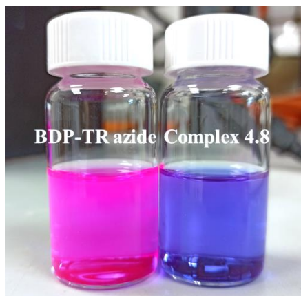
Figure 4.11: Visible colour change from BDP-TR azide to complex 4.8 in CH 2 Cl 2 solvent
