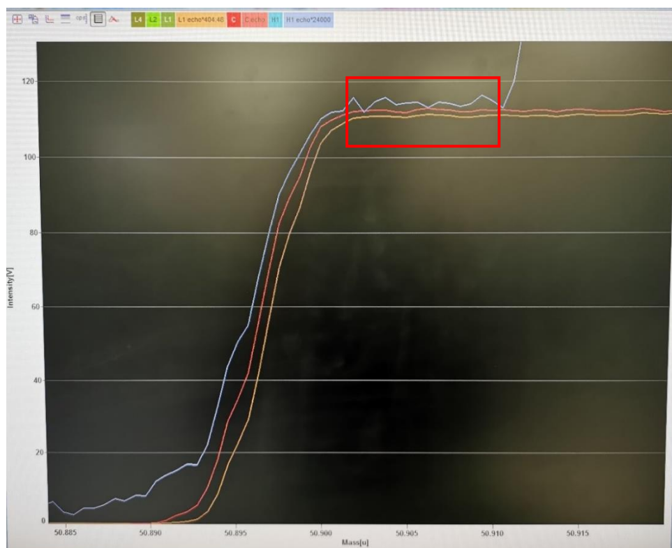
Figure 2.10: Screenshot of mass scan from Neptune software during V isotope measurement. The red box shows the ideal position on the mass 51 plateau to minimise interferences when analysing V isotopes.
