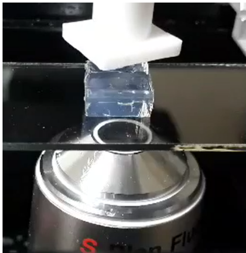
Figure 4.1: Photograph of the compression device located above the objective of an inverted microscope imaging a hydrogel sample.
