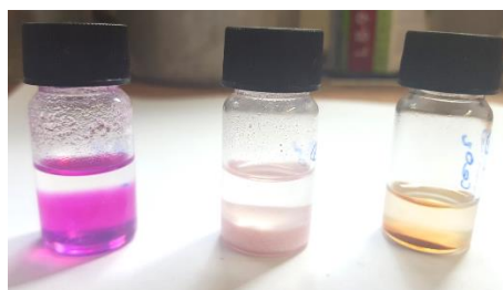
Figure 35: Photograph showing the colour change on exposure of different oxide supports to and adsorption of the Hammett indicator methyl red in toluene solution: silica (left); titania (middle); ceria (right)
