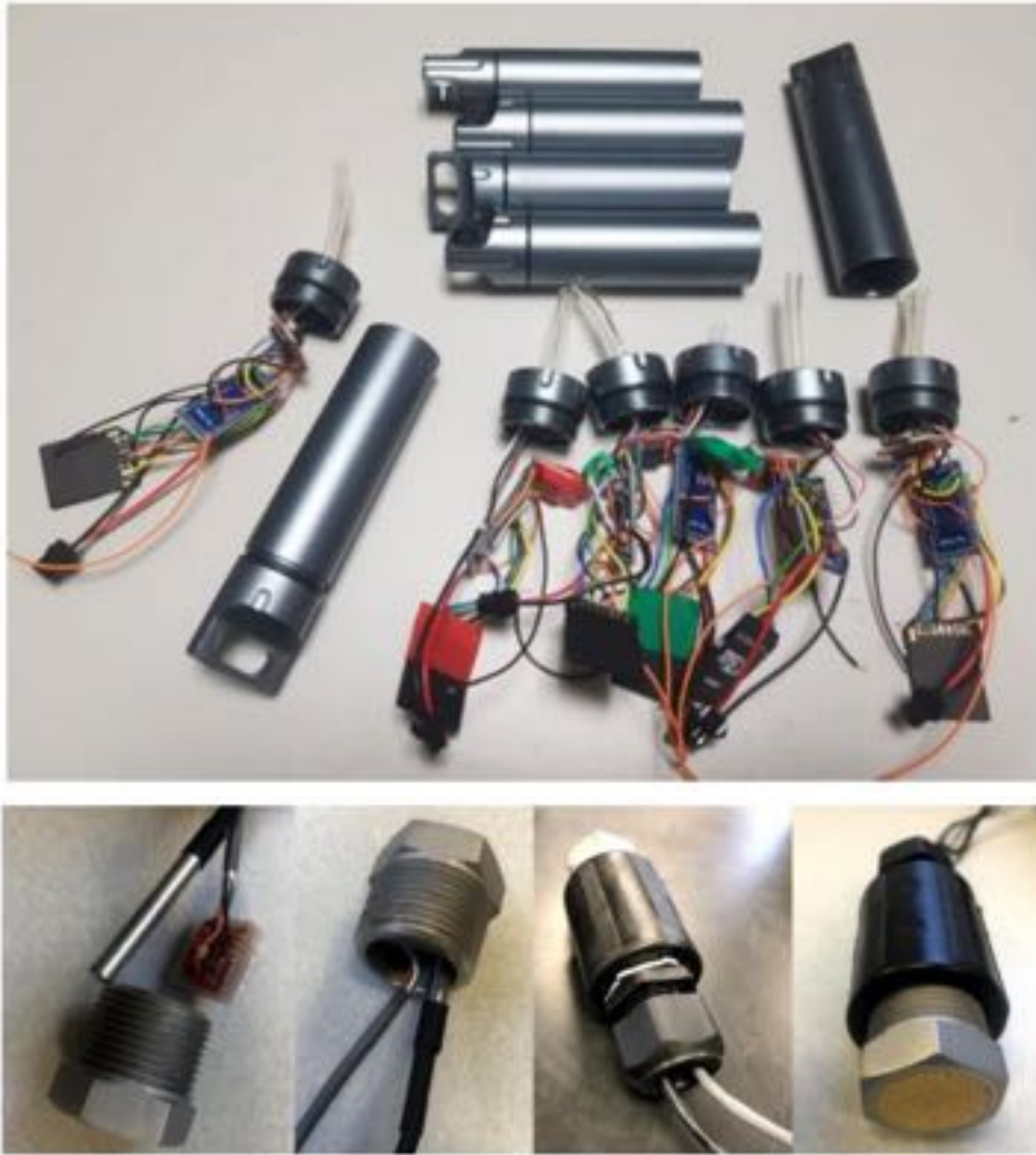
Figure 1.20: Examples of DIY pressure transducers. (Top)- Freestation pressure transducer with integrated pressure monitor and Arduino and (Bottom)- EnviroDIY pressure sensor only hidden inside a bolted pipe (Horsburgh et al. , 2019b; Chan et al. , 2020)
