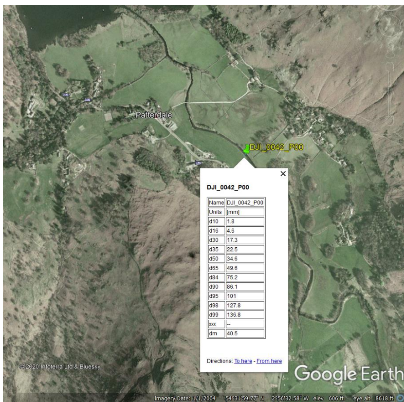
Figure 3.16 Grain size fraction results exported as KML file for display on Google Earth.
