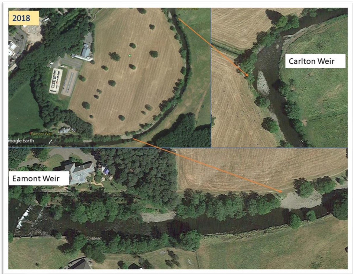
Figure 6.20 Illustrate that the Carlton weir was removed (in 2016), and geomorphic changes were observed in 2018.
