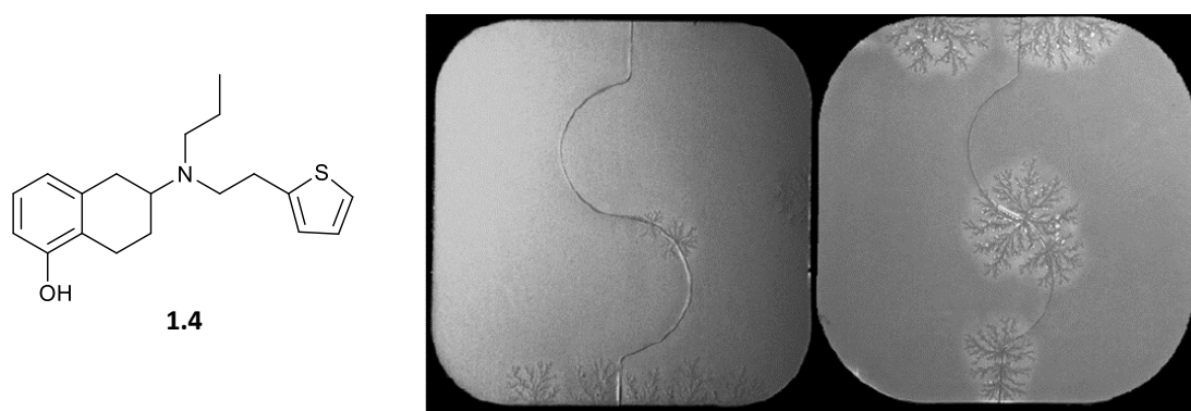
Figure 1-8. Form 2 of Rotigotine crystallising from Neupro patches which resulted in the withdrawal of Neupro patches from the market. Image adapted from reference 111.
