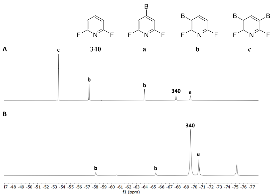
Figure 61: Crude ^{19}\text{F} -NMR spectrum in the borylation of 2,6-difluoropyridine using (A.) \text{B}_2\text{Pin}_2 and (B.) \text{B}_2\text{eg}_2 .
