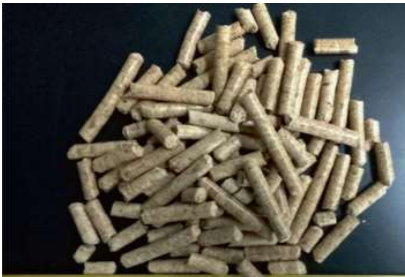
Fig 8-2: A typical pellets sample for use in a gasifier (Maguyon-Detras et al. , 2020)
