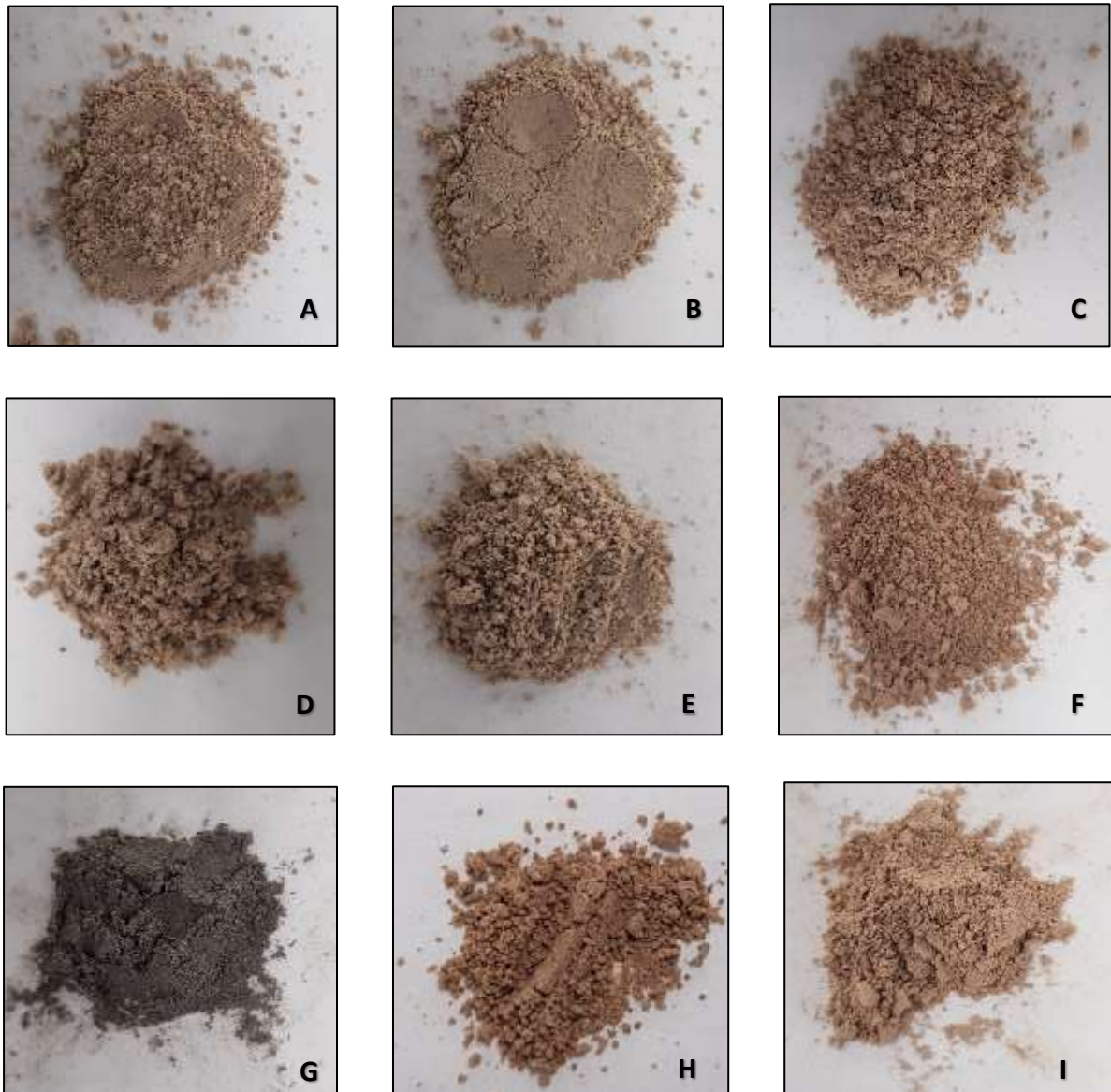
Fig 7-3: RSA (silica) preparation from (A: CSWW-L RS; B: CSTL-L RS; C: Water-L RS; D: Untreated-PT RS; E: HCl-PT RS; F: PE-PT RS; G: Raw RS; H: NaOH-PT RS and I: Digestate from hydrogen reactor)
