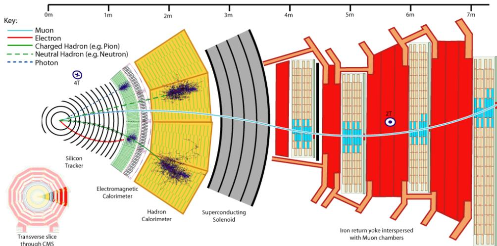
Figure 1.1: A cross-section of the CMS detector system at the LHC.
