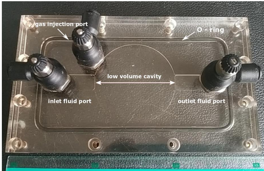
Figure 8.18. Second flow cell device. Thin base and top units, significantly reduced volume in the main cavity, repositioning of inlet and outlet ports for fluid flow and gas injection. The shape of the injection ports is changed; cylindrical ports are replaced.
