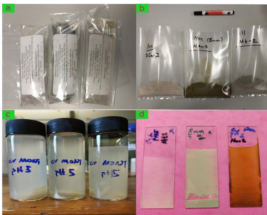
Figure 3.9. Sourced clays from the CMR (a), ground clays (b), montmorillonite clay suspensions before sonication (c), clay films (d).
