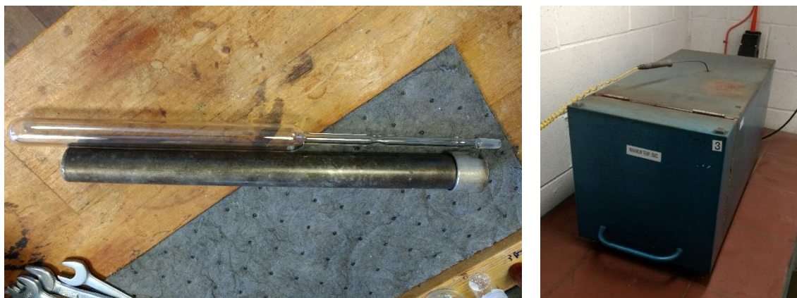
Figure 9.2. Carius tube (top-left) with steel container (bottom-left) and furnace (right)
