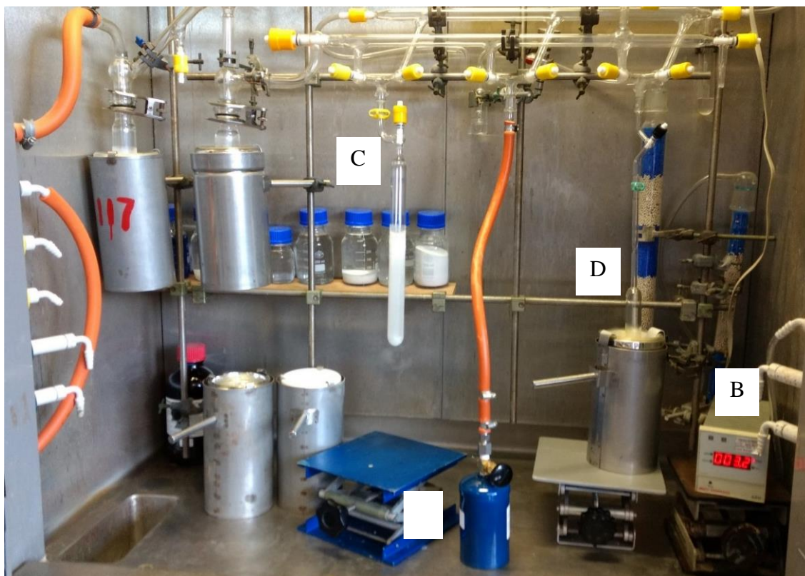
Figure 9.1. Example of a Carius tube being charged with gas
