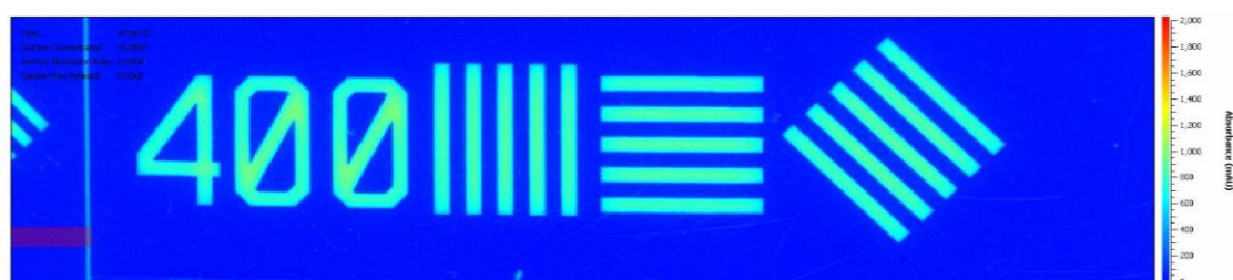
Figure 5.146 – Absorbance map using visible wavelength (520 nm) and the 400 grid. Shown in jet colour map and extracted from frame 24 of 591. Three distinct parts can be seen in the image: 1) 400 to show grid number, 2) vertical lines to test horizontal resolution, 3) horizontal lines to test vertical resolution and 4) diagonal lines for completeness.
