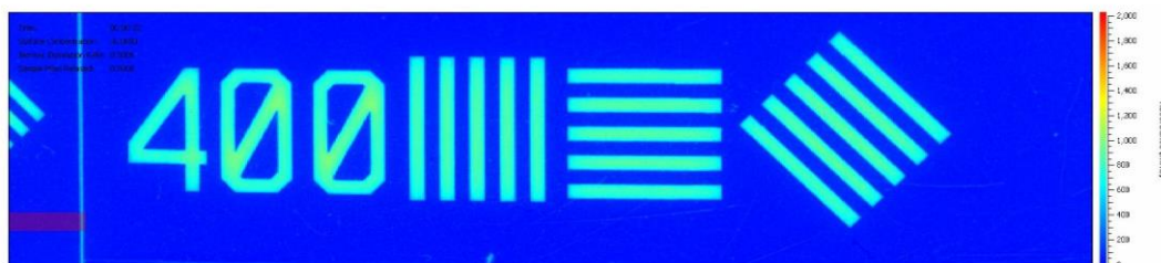
Figure 2.24 – Absorbance map using visible wavelength (520 nm) and the 400 grid. Shown in jet colour map and extracted from frame 24 of 591. Three distinct parts can be seen in the image: 1) 400 to show grid number, 2) vertical lines to test horizontal resolution, 3) horizontal lines to test vertical resolution, and 4) diagonal lines for completeness.
