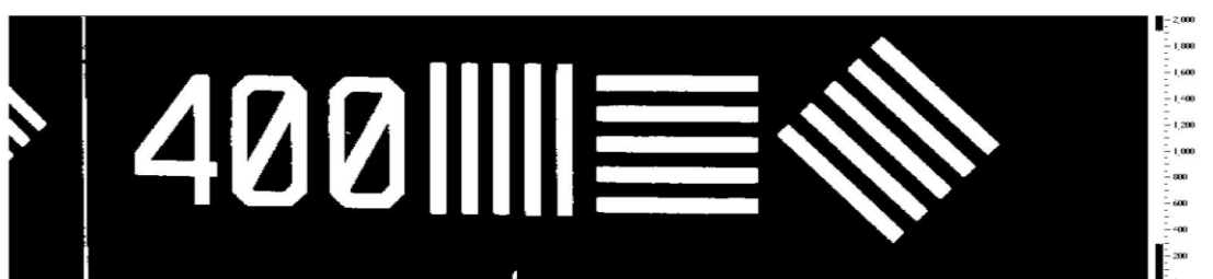
Figure 5.151 – Absorbance map using visible wavelength (520 nm) and 400 grid. Converted from Jet colour map to grey scale and then to black and white with a threshold of 100/255. Extracted from frame 24 of 591.
