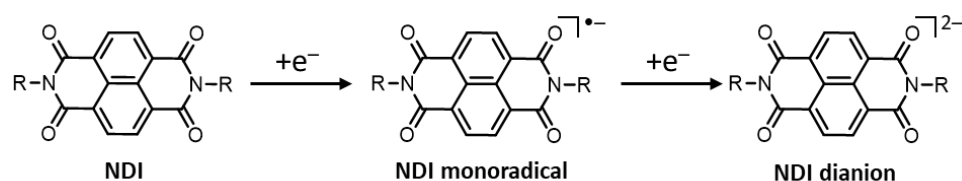
Scheme 1.1. Chemical structures of neutral NDI, which can be readily reduced to form an NDI monoradical which can be subsequently reduced a second time to form an NDI dianion.
