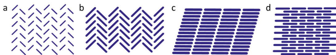
Figure 1.5. Molecular packing motifs of planar aromatics. a) herringbone packing (face-to-edge) with no significant \pi - \pi overlap, b) herringbone packing with \pi - \pi overlap, c) 1D lamellar packing and d) 2D lamellar packing.
