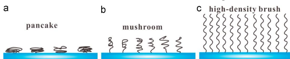
Figure 1.13: Diagram showing the variations in adsorption to solid surfaces of polymers with different monomer sequences. Reprinted with permission from reference. 193 Copyright Elsevier (2020)
