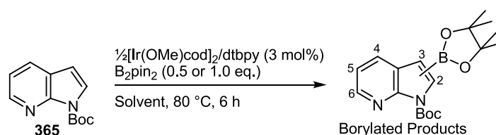
Figure 176 - Solvent screen for C-H borylation of N -Boc-7-azaindole.
