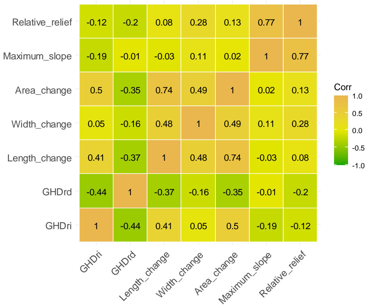
Figure 4.17: Correlation matrix for gully drivers. Effects of maximum slope and relative relief of gully head on changes in gully dimensions are small. GHDri = Gully head distance from rivers, GHDrd = Gully head distance from roads, Corr = Correlation legend.
