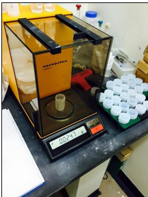
Figures 4.17 Weighing clean enamel samples in Teflon beakers (Left) followed by adding strontium spike solution (Right).
