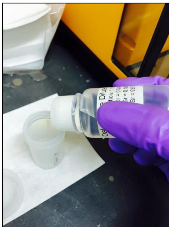
Figures 4.17 Weighing clean enamel samples in Teflon beakers (Left) followed by adding strontium spike solution (Right).
