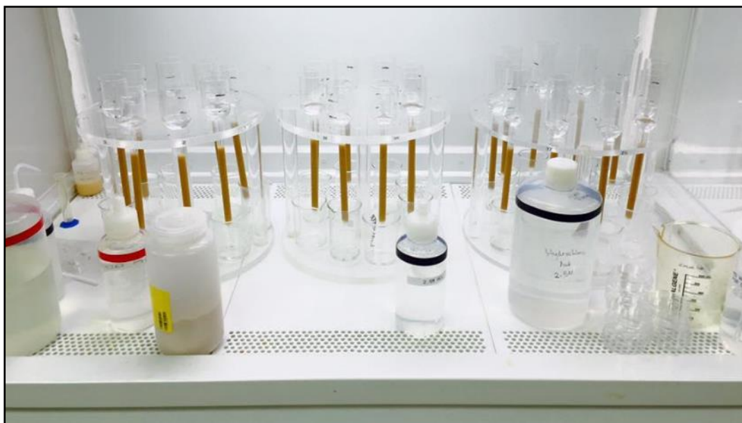
Figure 4.19 Eichrom AG 50w-X8 resin columns for column chemistry. Strontium samples were collected in the beakers below.
