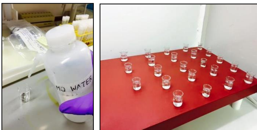
Figure 4.15 Ultrapure water added to enamel samples (Left) and samples on heated block in the laminar flow hood (Right).
