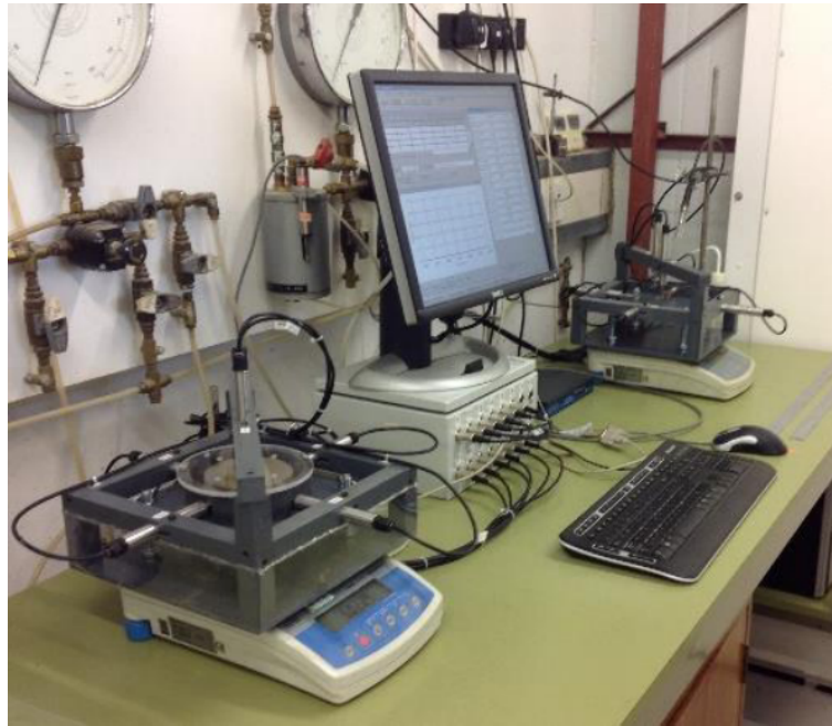
Figure 2.4: Durham SWRC high-capacity tensiometer equipment. Reproduced from Toll et al. (2015).
