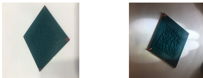
Figure 4.3: Watermark retrieval challenges due to illumination. Left: natural light. Right: uneven artificial light.
