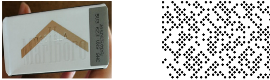
(a) DotCode on a pack of tobacco product for traceability. [125] (b) The up is ribbon-like; The bottom is square [123]
