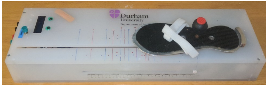
Figure 4. 1. Apparatus. The arm or leg could be moved along a linear track passively or actively. A metal stopper could be placed at locations along the track. Digital display showed movement time and a ruler was used to measure distance moved.
