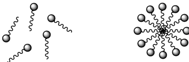
Figure 2.1: Free surfactant monomers in aqueous media (left) will undergo micellisation (right) at a critical concentration (CMC).
