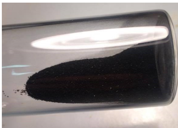
Figure 4.14: Product after mixed lamellar >95% sulfuric acid phase synthesis with 2.8 g >95% sulfuric acid and 0.8 g xylose solution at 80 °C. A hard shiny black powder can be seen. Product is pictured in a 14 ml squat vial.
