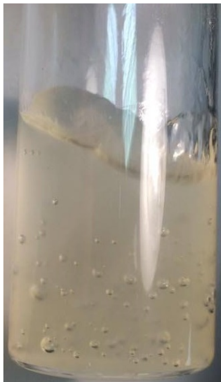
Figure 4.12: Upon combining Brij ® 30 (6 g) and >95% acid (2.4 g), a homogeneous lamellar phase gel is formed. Slight discolouration is seen. Gel is pictured in a 28 ml squat vial.
