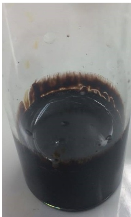
Figure 4.18: Upon addition of fuming sulfuric acid (2.4 g) to Brij ® 30 (6 g), the gel turned immediately black, indicating complete surfactant degradation. Gel is pictured in a 28 ml squat vial.
