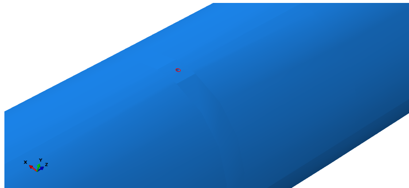
Figure 4.10: Hole type defect used for simulations.
