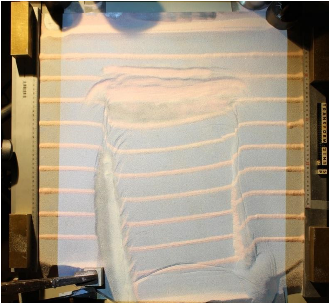
Figure B8 – Top view of Experiment 2 at the end of oblique rifting, without interpretation.
