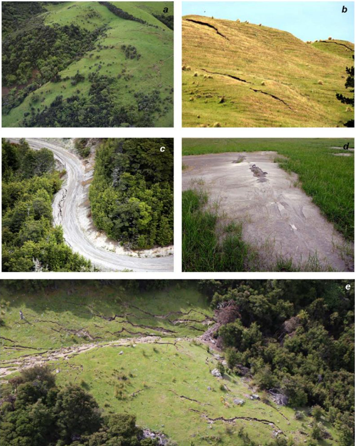
Fig. 3.12a-e: Sightings of ground cracking throughout the Kaikoura region documented by Jibson et al. (2018) during immediate post-earthquake field reconnaissance. Full credit to Jibson et al. (2018) – reference in bibliography.
