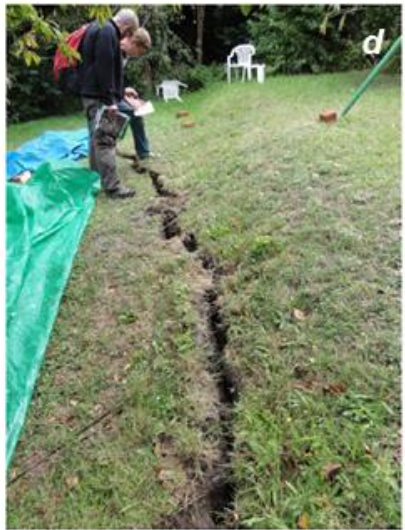
Figs. 3.08a-f: Examples of ground cracking in Christchurch which manifested during the Canterbury Earthquake Sequence in 2010-11. Documented by Dellow et al. (2011). Full credit to Dellow et al. (2011) – reference in bibliography.
