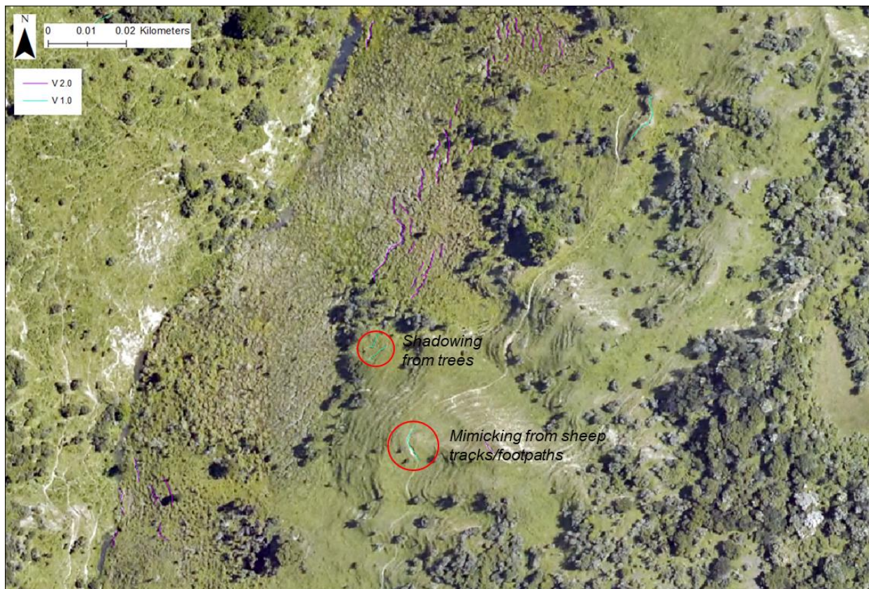
Fig. 4.05: Examples of error sources (highlighted) faced with when mapping co-seismic ground cracks by visual interpretation. Erroneous ground cracks were removed during quality checking, and as such some cracks from V 1.0 have been removed (highlighted in light blue, as have not been overlaid by V 2.0, the quality checked dataset). Note that density (Figs. 4.04a-b) was also a considerable source of error.
