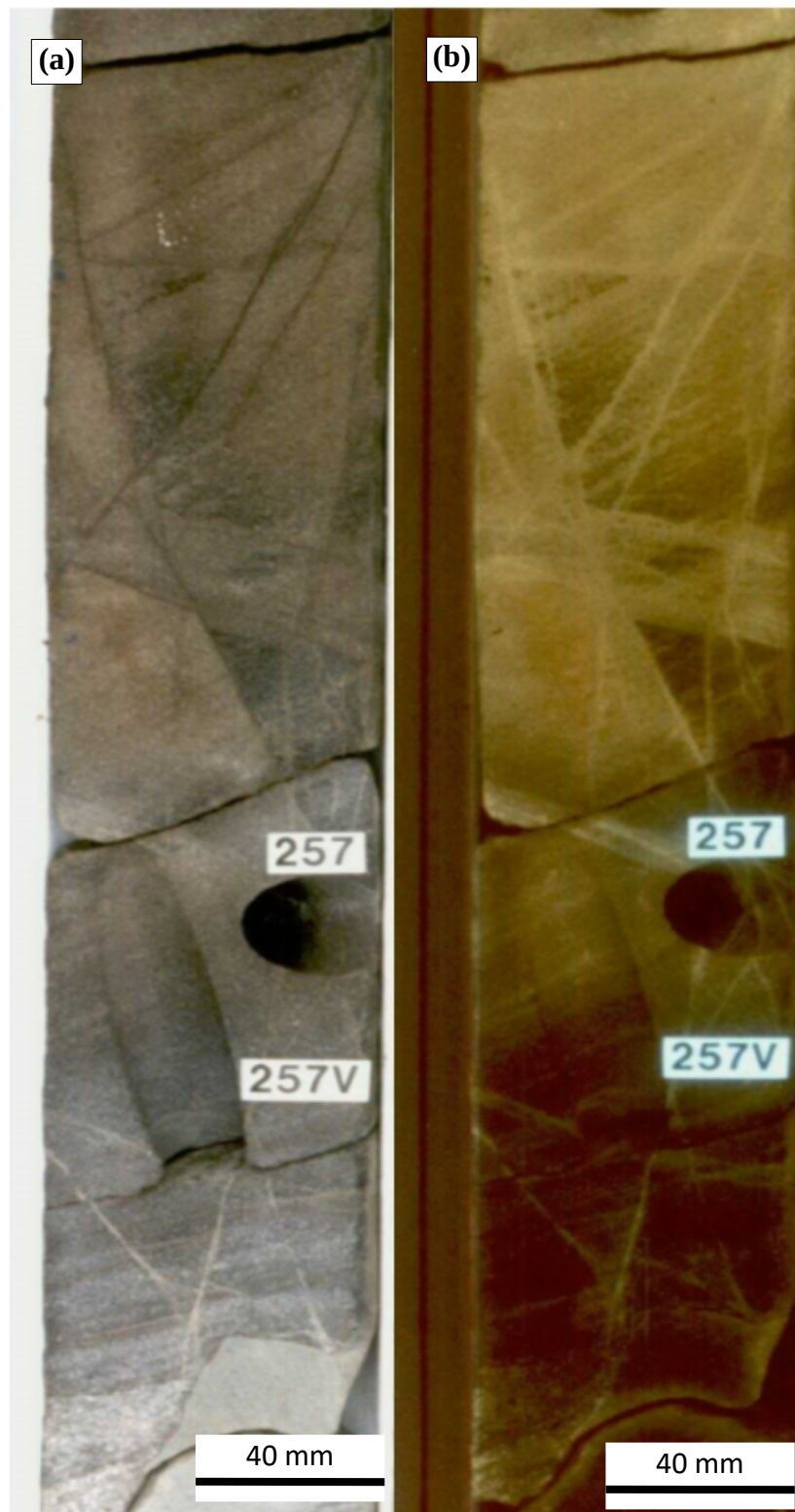
Figure 2.22: Section of core with (a) photographed under white light and (b) photographed under UV light. A difference in fluorescence is observed across a set of steeply dipping deformation bands possibly indicating that the deformation band acted as a baffle during hydrocarbon migration [well 22/29-2 (4173.99 – 4174.32 m MD/13694.2 – 13695.3 ft. MD)].
