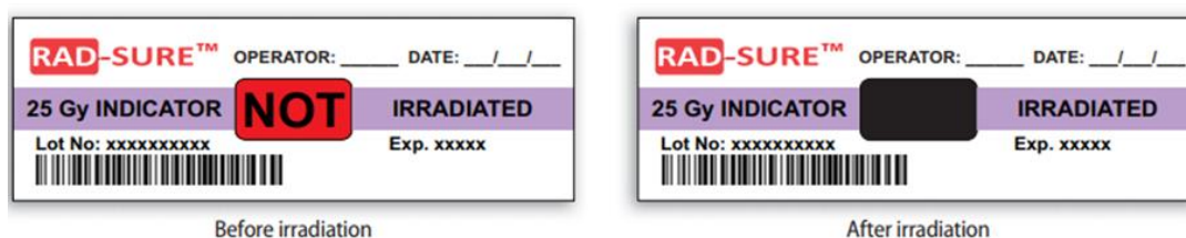
Figure 1.40. Radiochromic film labels used for irradiation detection on blood bags. Figure reproduced from reference 232.
