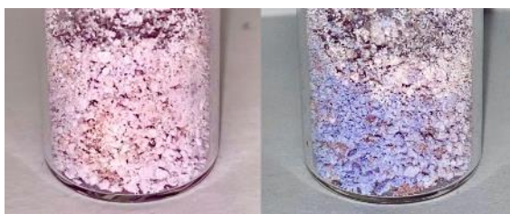
Figure 5.12. Both sides of a glass vial containing \text{BiCl}_3 and PCDA in a 1:2 ratio and placed under a shelf in the lab for approximately six hours shows a colour change when exposed to ambient light.
