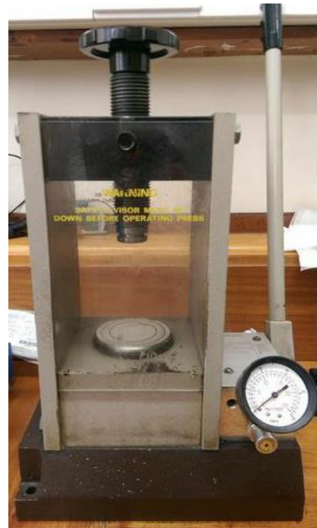
Figure 8: Specac Hydraulic Press with manual hand-pump and pressure gauge.
