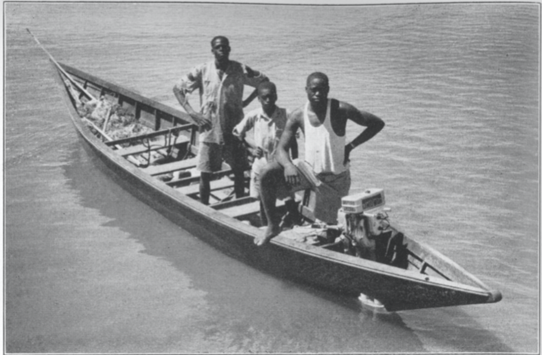
Figure 31: B.G. Kinloch, 'The "new look" in fishing canoes – Kabalega-built boat specially designed for use with an outboard motor'. 848
