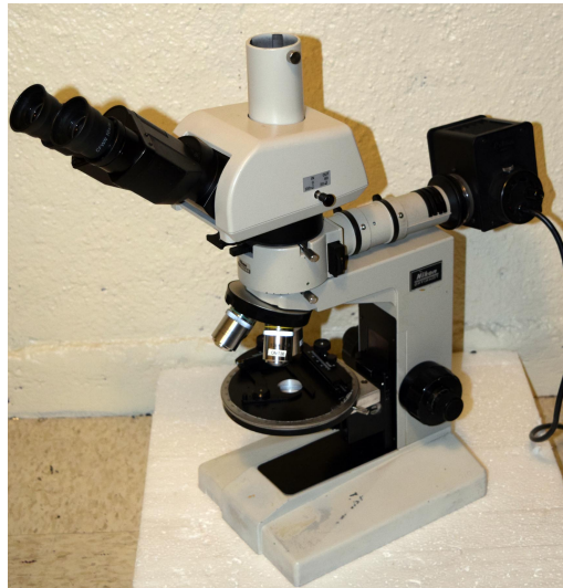
Figure 4.8: Original Nikon microscope similar to the one used as a base for the homemade MOKE Microscope.
