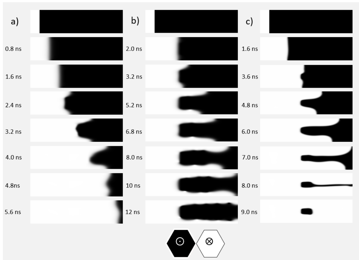
Figure 7.7: Colour representation of m_z , measured after the injection positive current pulses. Time scale in the left-hand side. SOT current-driven domain wall motion a) J = 5 \times 10^{12} A/m 2 complete switching of the strip b) J = 3.8 \times 10^{12} A/m 2 , the current could not overcome the PMA of pillar. c) J = 3.8 \times 10^{12} A/m 2 making the pillar smaller and applying a small current in the opposite direction enables to just have the pillar. Colour wheel at the bottom representing the magnetic moment direction.
