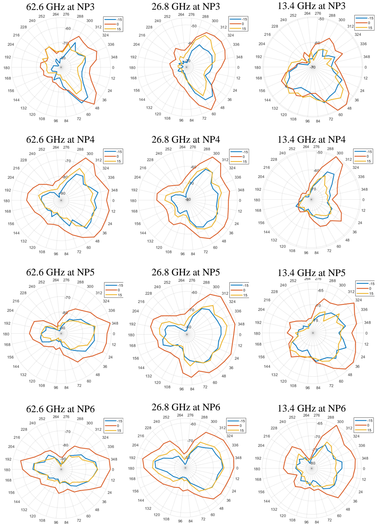
Figure 5-30 Polar plots of the received power versus azimuth angles at the strongest three elevation angles for all bands
